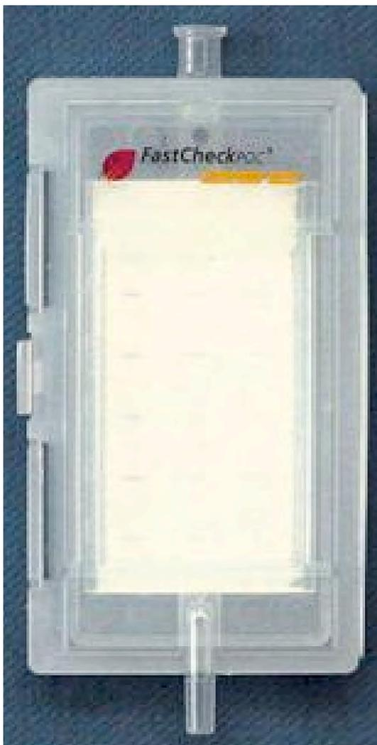
**Figure 2:** The fast allergy test housing holds the test membrane with allergens and controls inside a flat incubation chamber. A latch keeps the lid in a half open position during sample incubation and assures tight fitting of the lid when closed. The device is closed completely before conducting washing steps and substrate incubation. Washing solution and substrate are added through the upper Luer lock using a syringe.
